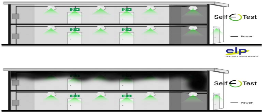
Fig. 7. Smoke propagation in the interior of a building Source: https://www.elp.uk.com/ (with modifications)
