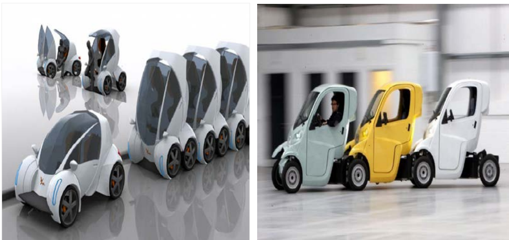
Fig. 4. Small vehicles: a) MIT's Stackable City Car, Source: https://inhabitat.com/transportation-tuesday-mits-stackable-city-car/ , b) Stackable cars - Light weight L category electric vehicle that can be stacked together to gain space – to be developed in the Easily Distributed Personal Rapid Transit (ESPRIT) project, Source: ESPRIT project http://www.esprit-transport-system.eu/
