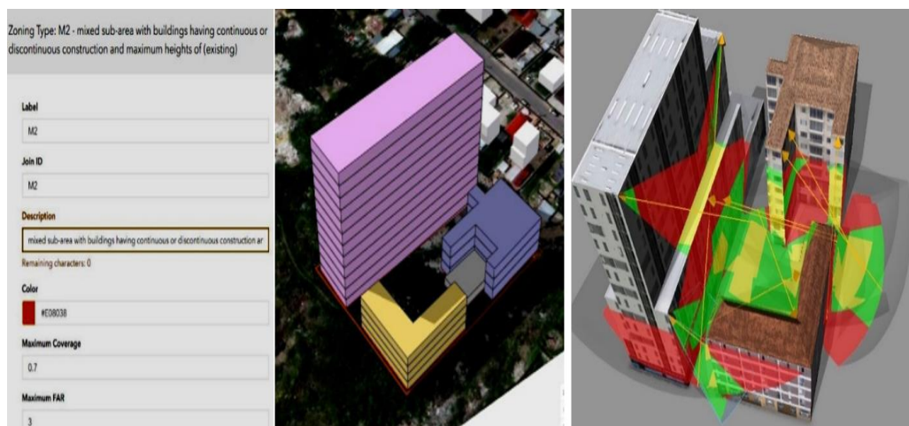
Fig. 4. Spatial Planning in ArcGIS Urban (left side) and Scenario of the Surveillance Cameras Location in the Projected (right side in CityEngine) (adapted from [8])
