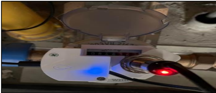
Fig. 1. Example Water Meter Monitoring Kit setup Source: www.watermeterkit.nl
