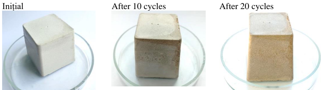
Fig. 16. Resistance to repeated freeze-thaw cycles specimens with walnut sawdust
