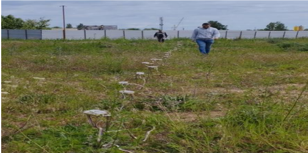
Fig. 8. Specialist performing an Electrical Resistivity Tomography with the electrodes placed linear array Source: INGEVO Engineering Evolution
