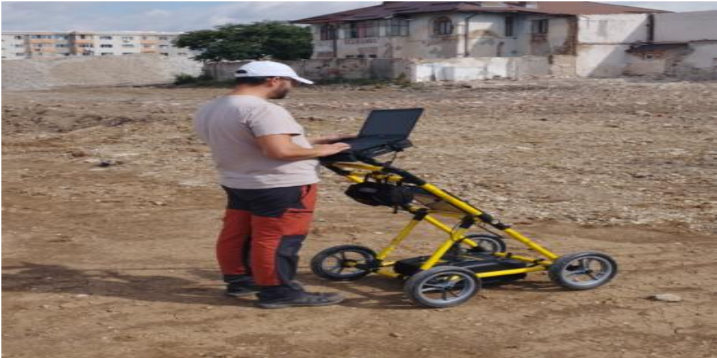
Fig. 9. Specialist scanning the land using a Ground Penetrating Radar Source: INGEVO Engineering Evolution
