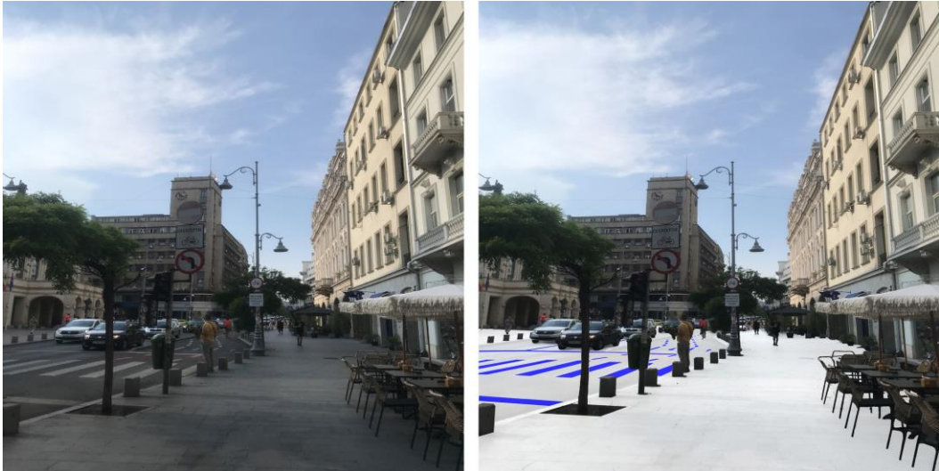
Fig. 4. Thermochromic pavement and asphalt on Calea Victoriei Street (and sidewalk). Bucharest (Romania)
