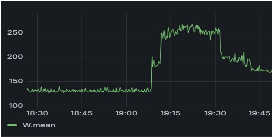
Fig. 5. Power consumption during Gemma 12B inference showing sustained elevation to 250 W over 20-minute execution.
